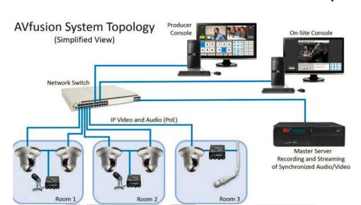
AVFusion synchronizes audio with video to enable recording & on-the-fly editing of A/V content.
