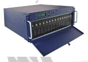
Veracity's ColdStore NAS array uses one-tenth of the power of comparable systems, is resilient to disk failure, and requires no disk rebuild process. Disks can be added "on the fly" and will automatically be incorporated into the array.
